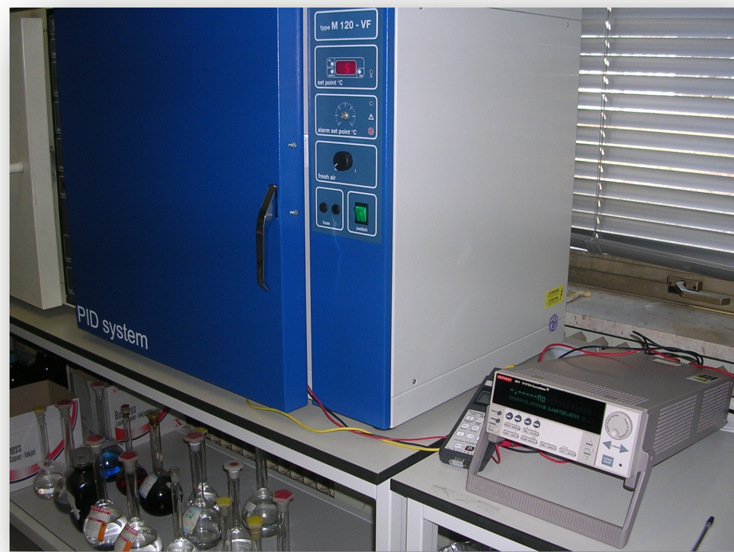
Figure 1 - Environmental chamber, temperature and resistance meter gauges used in the tests
